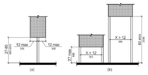
ABAAS Figure 307.3 Post-Mounted Protruding Objects
